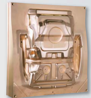
D2 forming die, coated with Duplex-Variantic work material: hot rolled 1.0335 steel.
